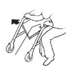
**BACK WHEELS** Large rear wheels should be inspected at least once a month to ensure proper tightness. If wheel wobbles or is loose, release lock nut and tighten axle bolt slightly. Test for proper tightness by leaning chair to one side and spinning adjusted wheel.
