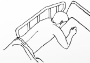
Entrapment between the rail and mattress
