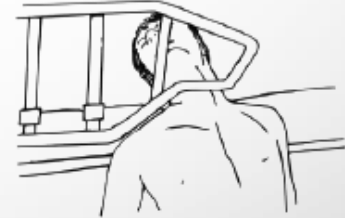
Entrapment under the bed rail at the ends of the bed rail
